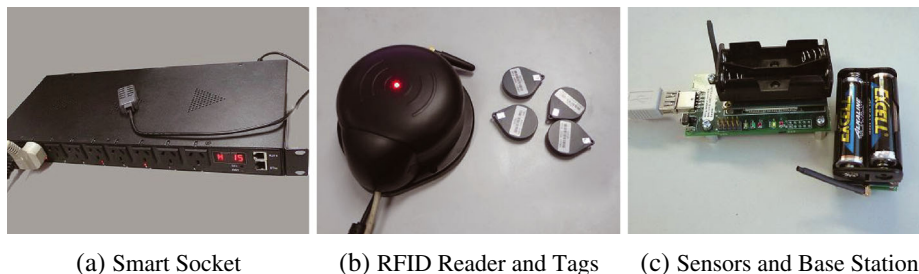
Figure 5. Smart objects and devices in a remote appliance management system. (a) Smart socket, (b) RFID reader and tags, and (c) sensors and base station.
