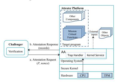
Fig. 3. Software layout of the attestation scheme
